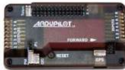
Figure 14: Microcontrollers used in drones and rovers
